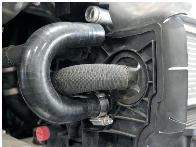
11. Now disconnect the water pipe (passenger side) to the original radiator with the appropriate tool.
