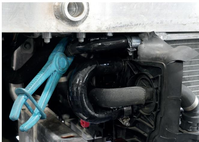
13. Now connect the other end of the enclosed silicone elbow 180 ° to the **free connection of the original cooler (1)** and fix it with the supplied hose clamp.
