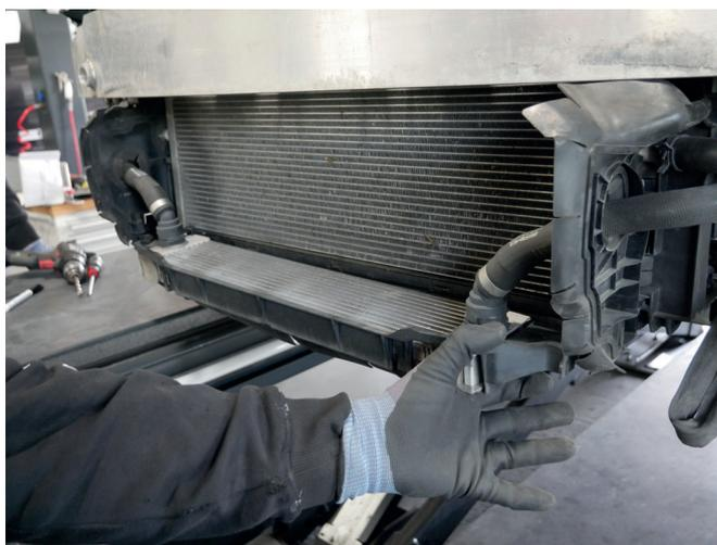
3. Now loosen the retaining clips of the plastic side cover of the standard water cooler. It is best to use a flat-head screwdriver or similar. These then also pull out of their attachment position.
