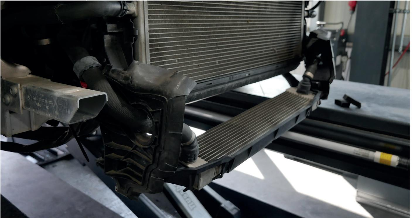
5. Align the HF-Series Auxiliary Water Cooler as far as possible towards the engine compartment.
