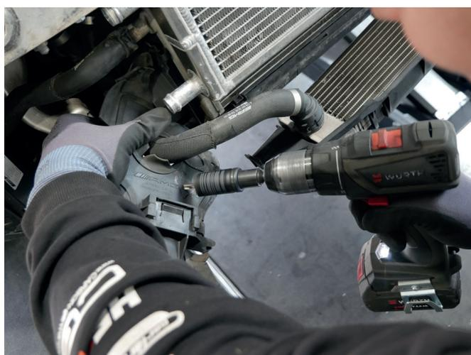
9. Now assemble the plastic side parts and the original water cooler in the reverse order and check again the free movement of the components, especially in the area of the connections of the additional water cooler.
