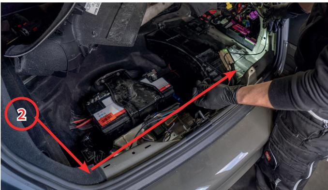
Instructions for routing the wiring harness on the driver's side.
