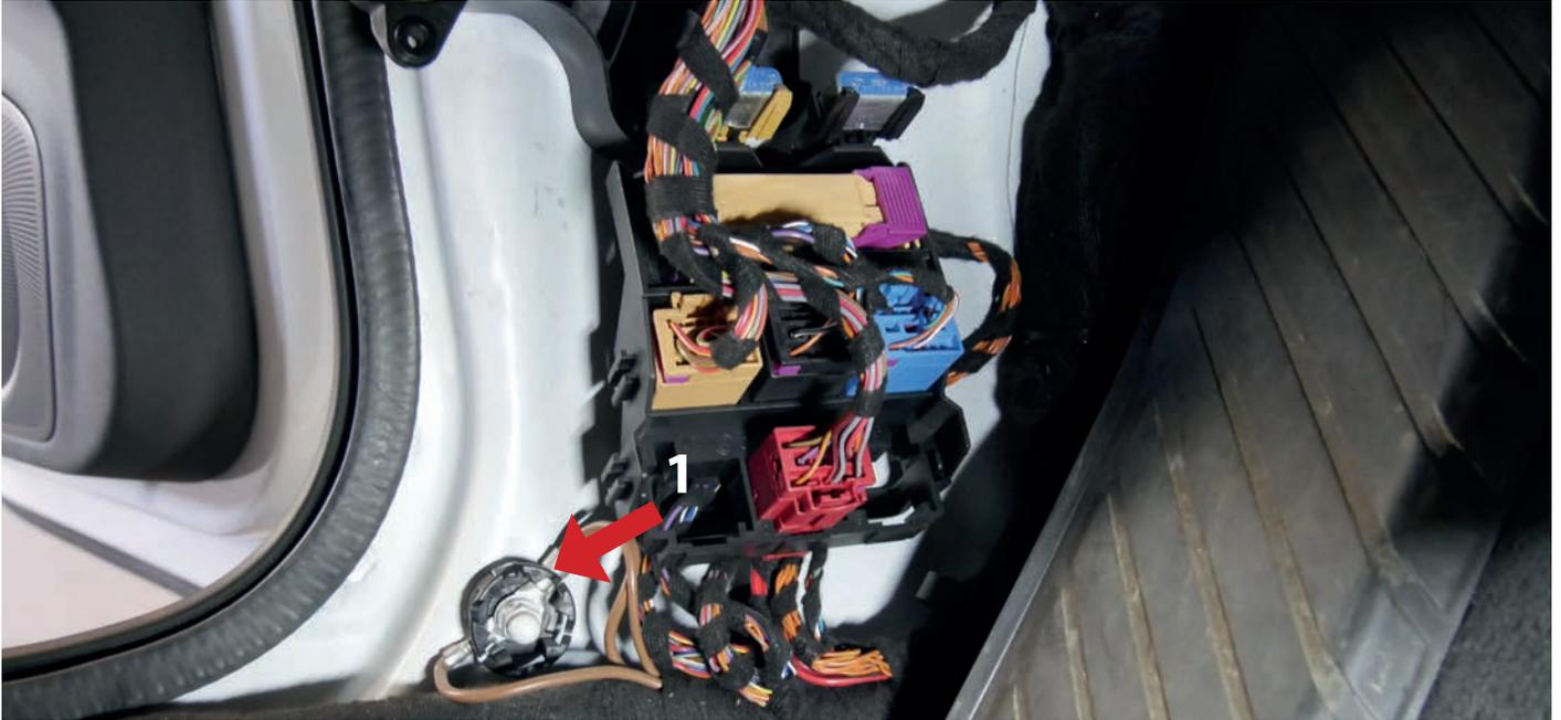
4. At the plug you can find the Can Bus cables (1)
