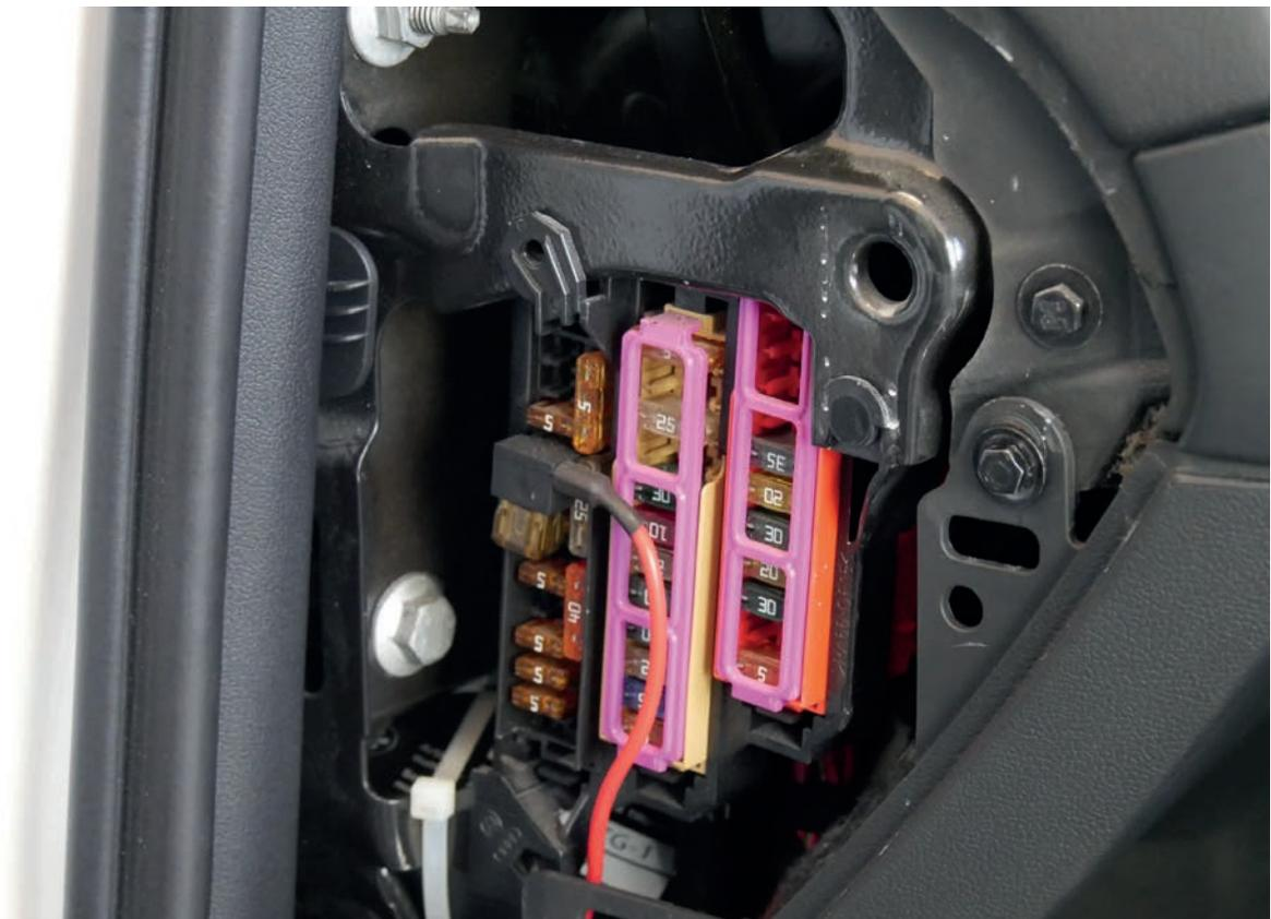
3. At the area of the side sill you can find the **mass (1)**, where you can connect the mass supply with the Bull-X Tronic.
