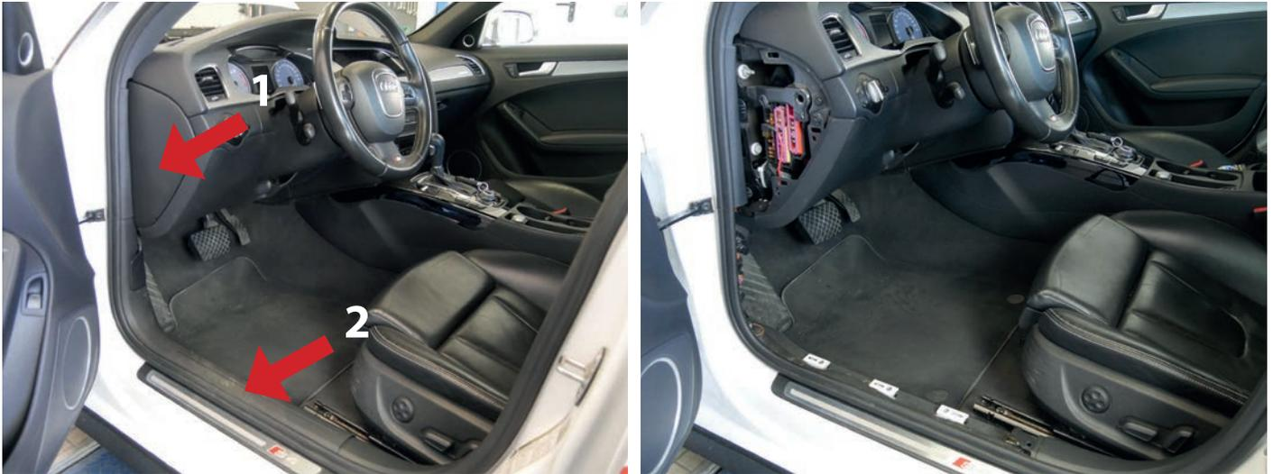
2. You can find the fuse box under the cover of the dashboard, where you can find the needed 12 +V. Measure the cables at various points until you find the needed 12 +V and connect this cable with the Bull-X Tronic cable.
