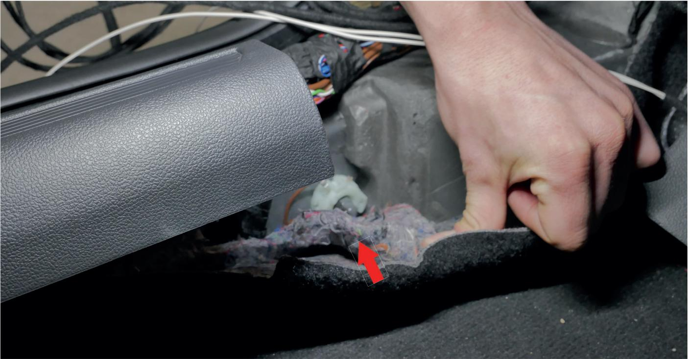
4. To pick up the ignition plus, locate the 20A fuse in slot F55 in the fuse box of your vehicle. Remove the fuse, insert the supplied fuse holder into the slot of the previously removed fuse and insert it into the fuse holder.
