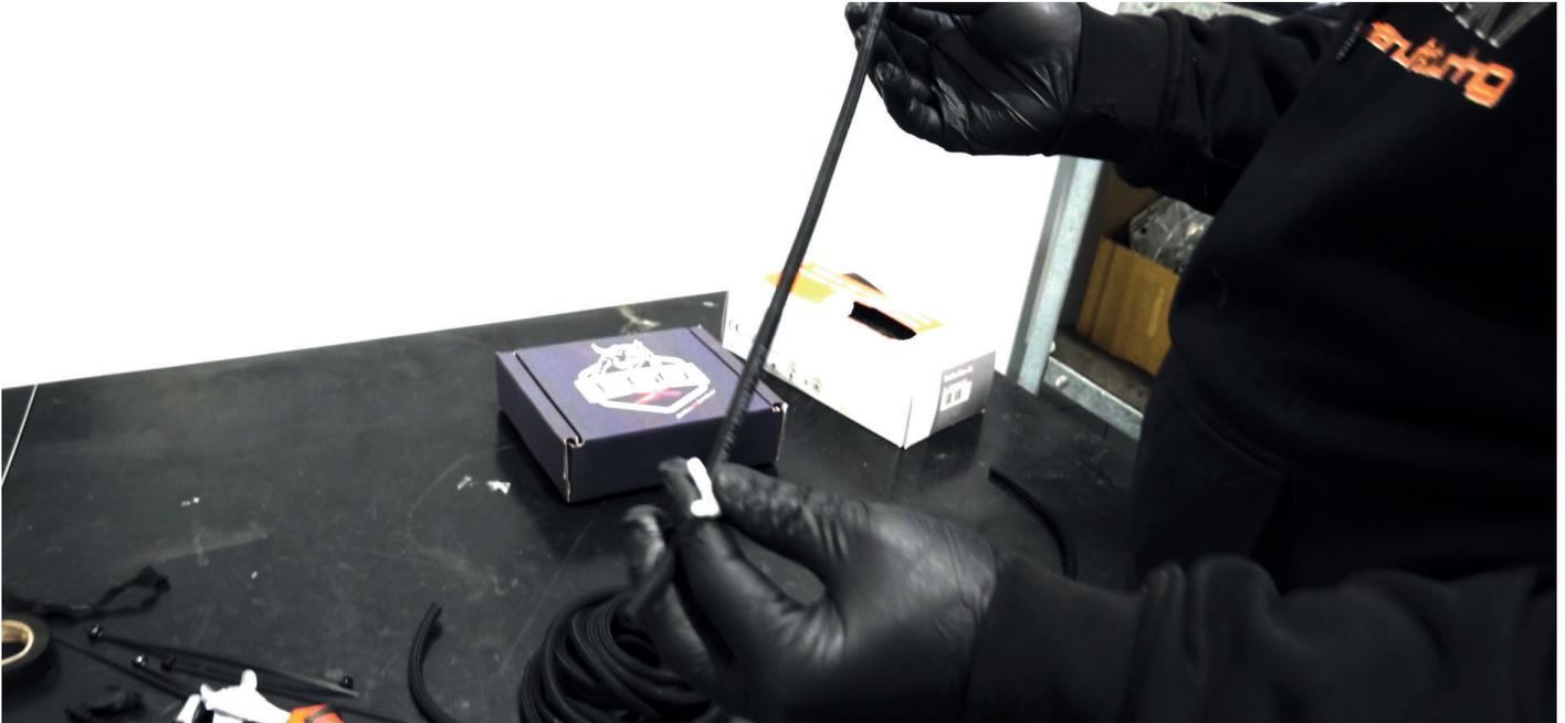
8. Then insert the check valve onto the other end of the long length of tubing. Pay attention to the direction of the arrow on the check valve as well as to the instructions in the „General Installation Instructions“.
