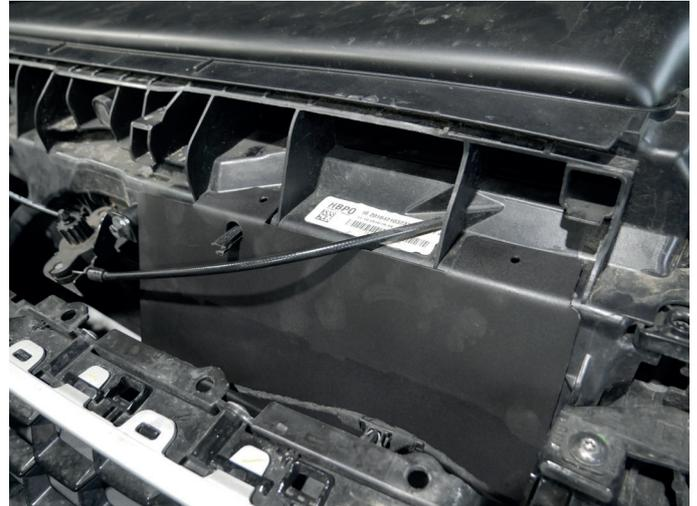
3. As positioned, hold one sheet at a time and drill through the holes in the retaining tabs into the vehicle's front mask using a 3mm metal or plastic drill bit. Pay attention to surrounding vehicle parts. Then fix the air baffles with the provided coarse thread screws.
