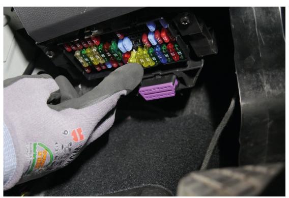
10. Insert the previously removed fuse into the fuse holder (this is included) and then insert it into the free slot of the previously removed fuse. Now you can use the red cable of the fuse holder (secured with 10 ampere) to connect the ignition plus of the Bull-X Tronic.
