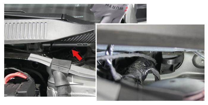
15. Route the cable in the water box of the vehicle towards the passenger side to the magnet valve (1).
