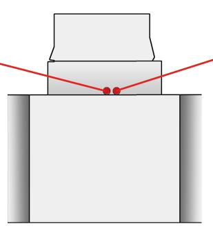
The second LED indicates the connection to the motor CAN bus. This has to flicker quickly, so it looks almost like it will light through.
