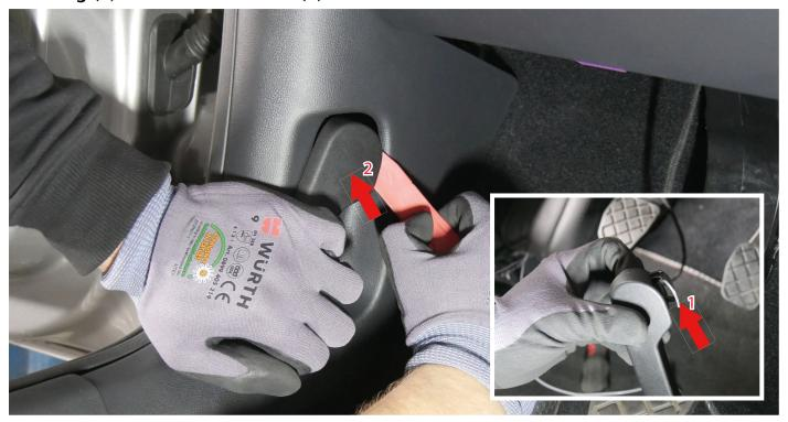
2. Now remove the release lever of the hood and remove the shown **blanking plug** (3).
