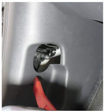
4. Use the plastic wedge to lever the paneling up so far that you can reach under with your fingers and, with a slight drag, pull the paneling towards the footwell. NOTE: When removing, the fixing pins often remain stuck in the bodypart. Pull out the pins and put them back into the paneling.
