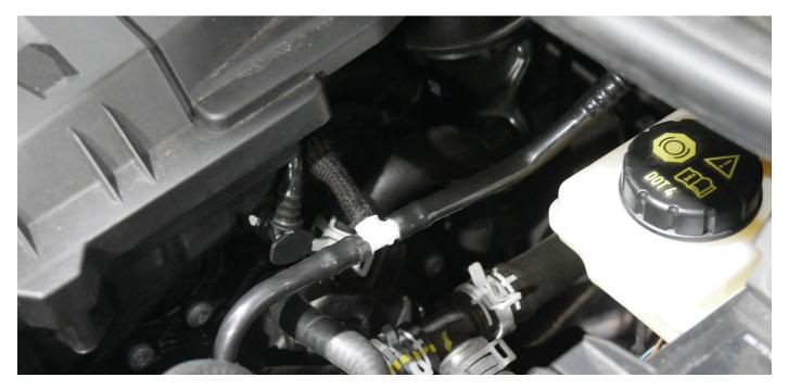
17. Now lay the vacuum line from the remaining connection of the magnet valve (2) in the direction of the underbody of the vehicle.
