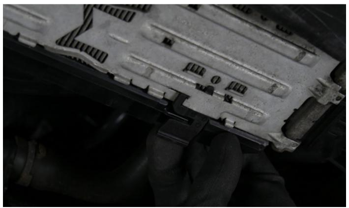
4. Now remove both T25 fastening screws on the left and right of the cooler and carefully pull the cooler down out of its holder.
