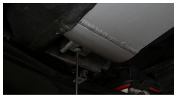
8. Now plug the charge air hoses onto the radiator connections and press them firmly into place. The hoses must be audible, snap into place all around and wiggle and pull, firmly connected to the cooler.
