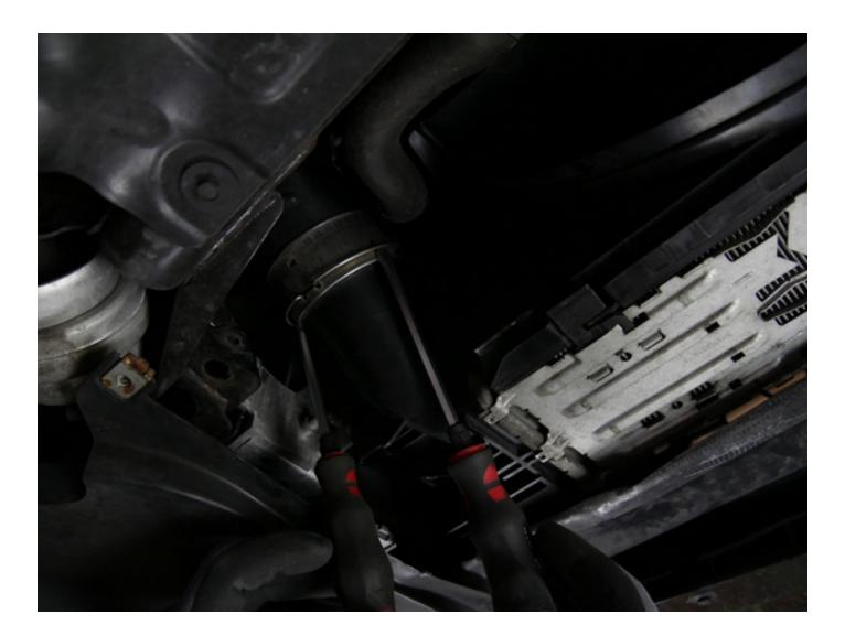
Note: Depending on the mileage of your vehicle, the clamps and the charge air hoses may be more or less stuck. If necessary, use a larger flat-blade screwdriver or similar to remove the hoses from the charge air cooler. But do not damage the charge air hoses or the clamps, as you will continue to use them.
