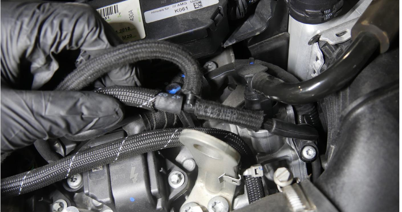
13. Mount the solenoid valve in a suitable place in the engine compartment and route the hose and cable in its direction.
