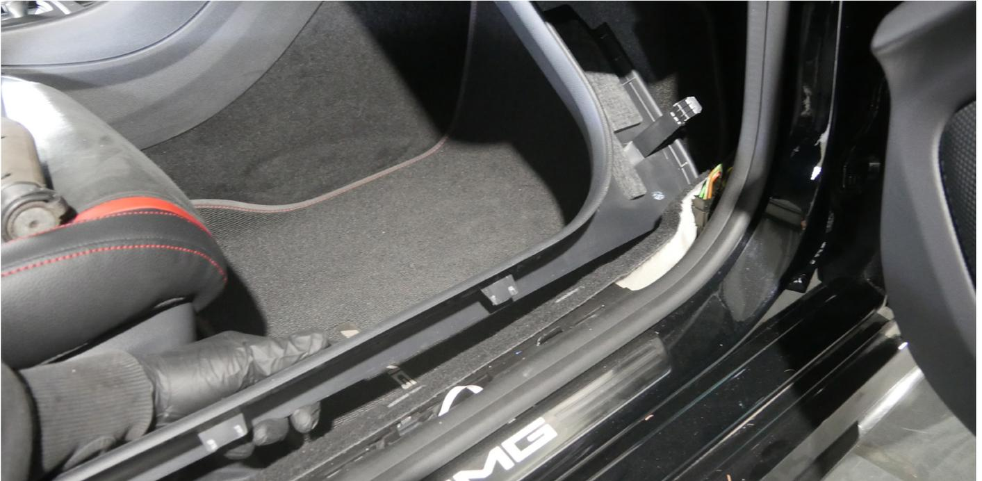
2. Disassemble the glove box by removing the mounting screws all around and fold down the carpet, behind it is the fuse box and Can Bus rail.
