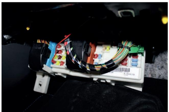
4. Next step is to pull the yellow-black cable and the black-white cable behind the dashboard in the direction of the obd-plug (marked with red arrow) . Therefor you have to remove the screw, which fixed the plastic cover. Connect the black-white cable (CAN high) with the cable on pin6 of the obd-plug (red-blue) and the yellow-black cable (CAN low) with the cable of pin14 of the obd-plug (red-white).
