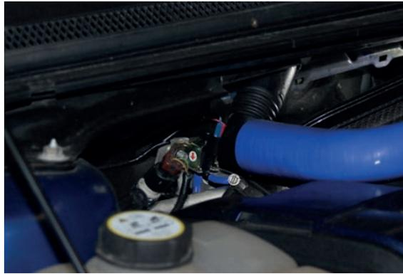
6. As the last step, connect the magnetvalve with the vacuum hose and the t-piece to the original vacuum hose as shown in the picture. Built in the glove compartment cover and the plastic cover on the left side of the dashboard.
