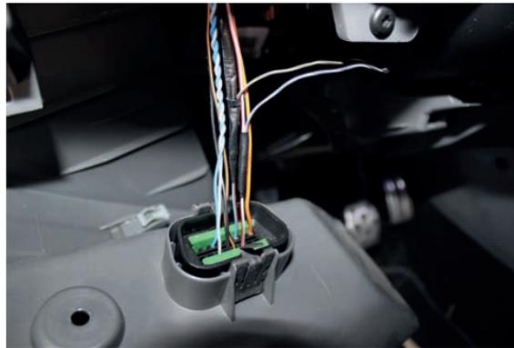
5. On the right side of the dashboard, you have to push or pull the plug with the purple and red-white cable from the Bull-X Tronic into the engine room and connect it with the magnet valve. Polarity doesn't matter.
