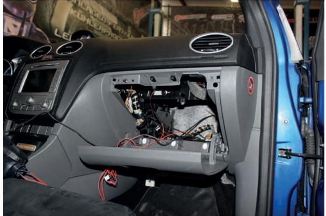
2. Fix the grounding cable (brown) with one of the screws above like on the picture below. Then place the Bull X Tronic unit in the shown position.
