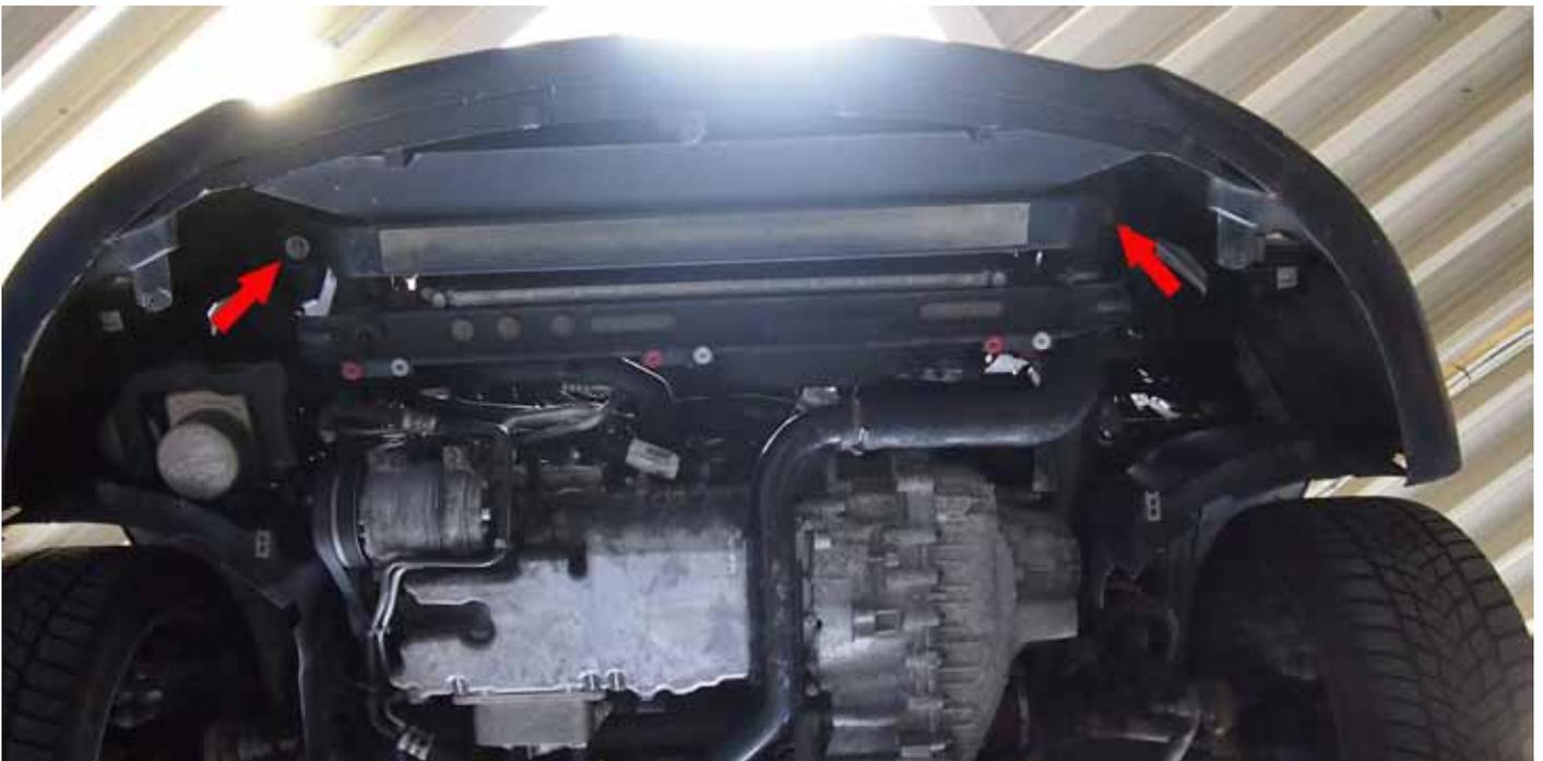
6. Carefully slide the old intercooler down at a slight angle.
