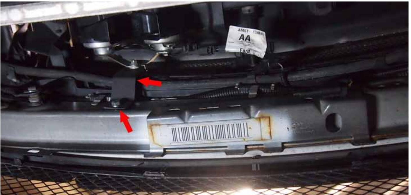
8. Screw the left and right retaining plates of the new intercooler to the original mounting points of the old intercooler between the front support and the support of the water cooler using a 10 mm nut or ring spanner.
