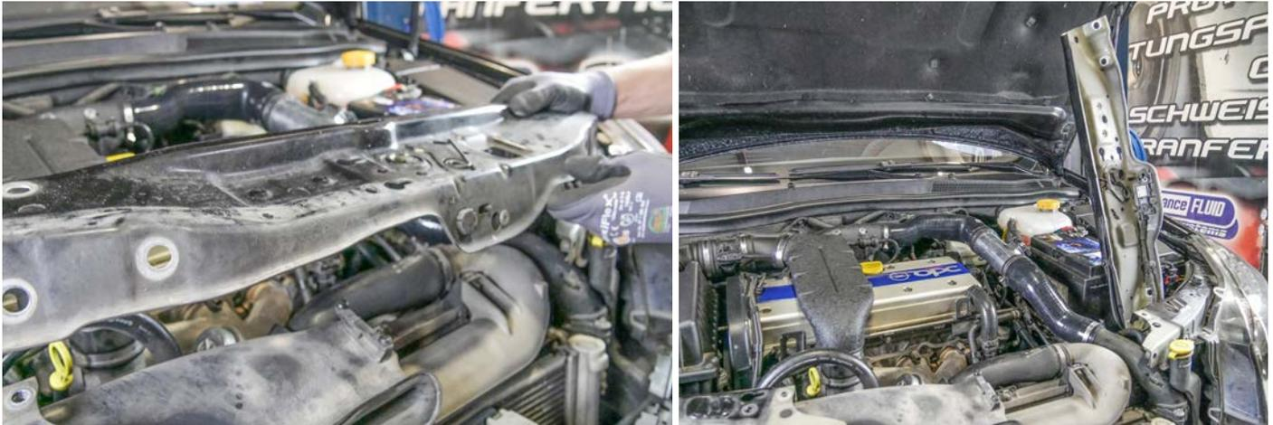
14. Release the clamp from the pressure pipe (with torx nut E8) and remove it.
