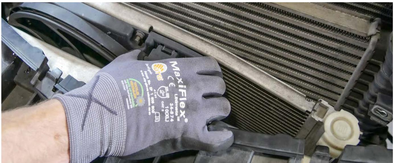
19. At the intercooler you have to remove the screws first (torx nut E8). After that you can put the intercooler a little bit upwards to get him out of the mount, and then just pull him down to release him totally from the car.
