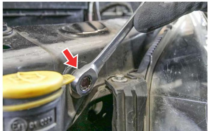
13. You can place the lock carrier aside now. Please not, that the lock carrier is also connected to cables that you need to remove first if you want to remove the carrier completely. We ajar him edgewise to the battery compartment. Beware of short circuit! Don't get close to the battery terminal directly.
