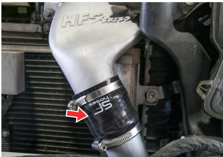
30. Attach the pressure pipe with the mapsensor pipe by using the supplied SF-hoses hump hose. Pull assembly down the clamps.
