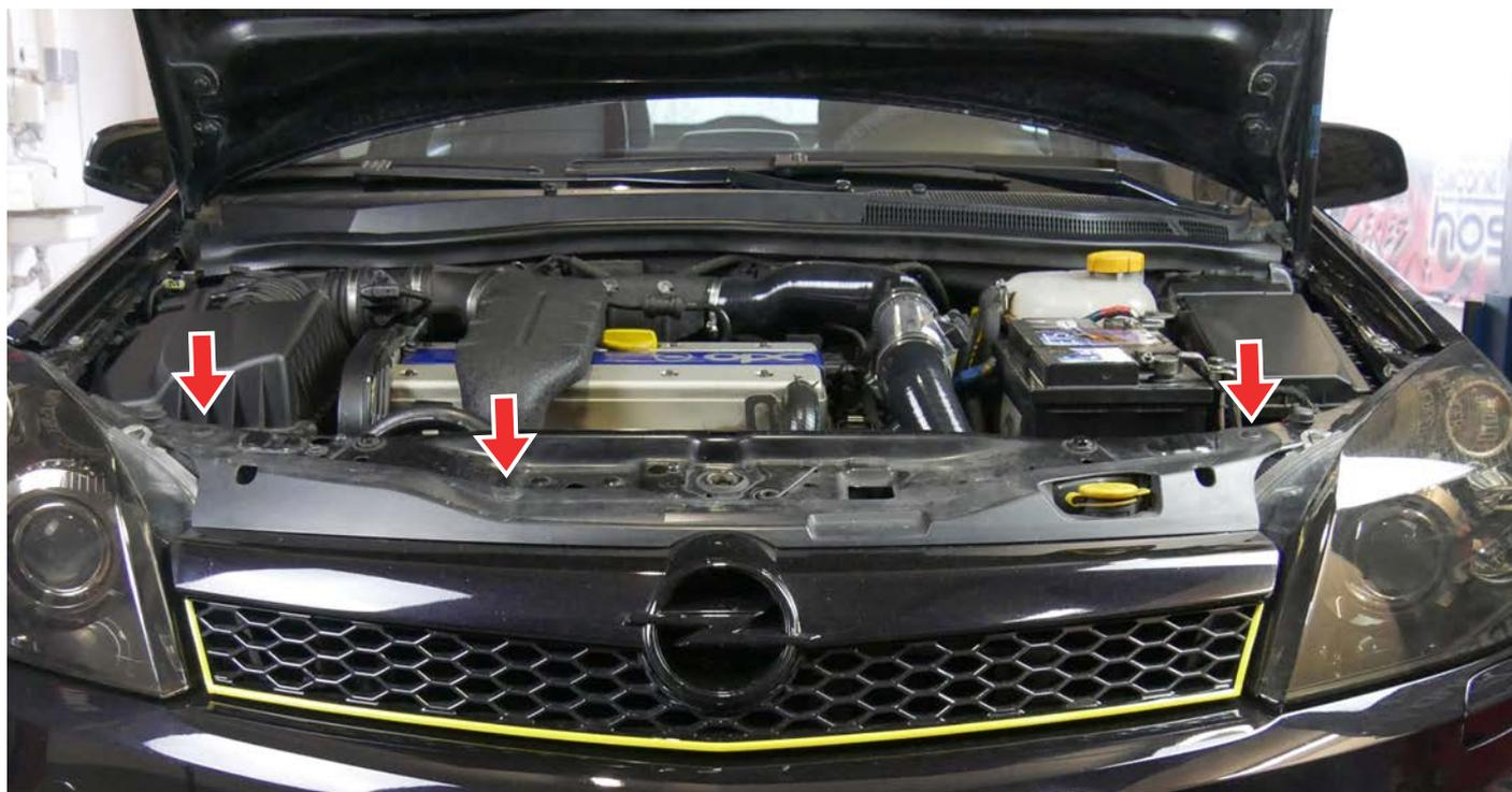
2. Press each pin down away ( For installation keep ) and pry the holder gently with a screwdriver out .
