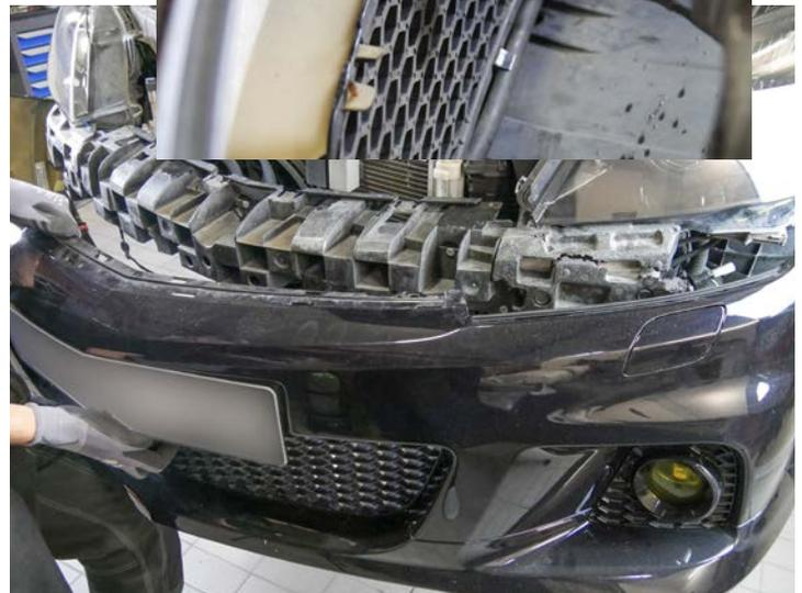
10. Release the screws on the lock carrier with a Torx T25 screwdriver to remove the intake of the air filter.
