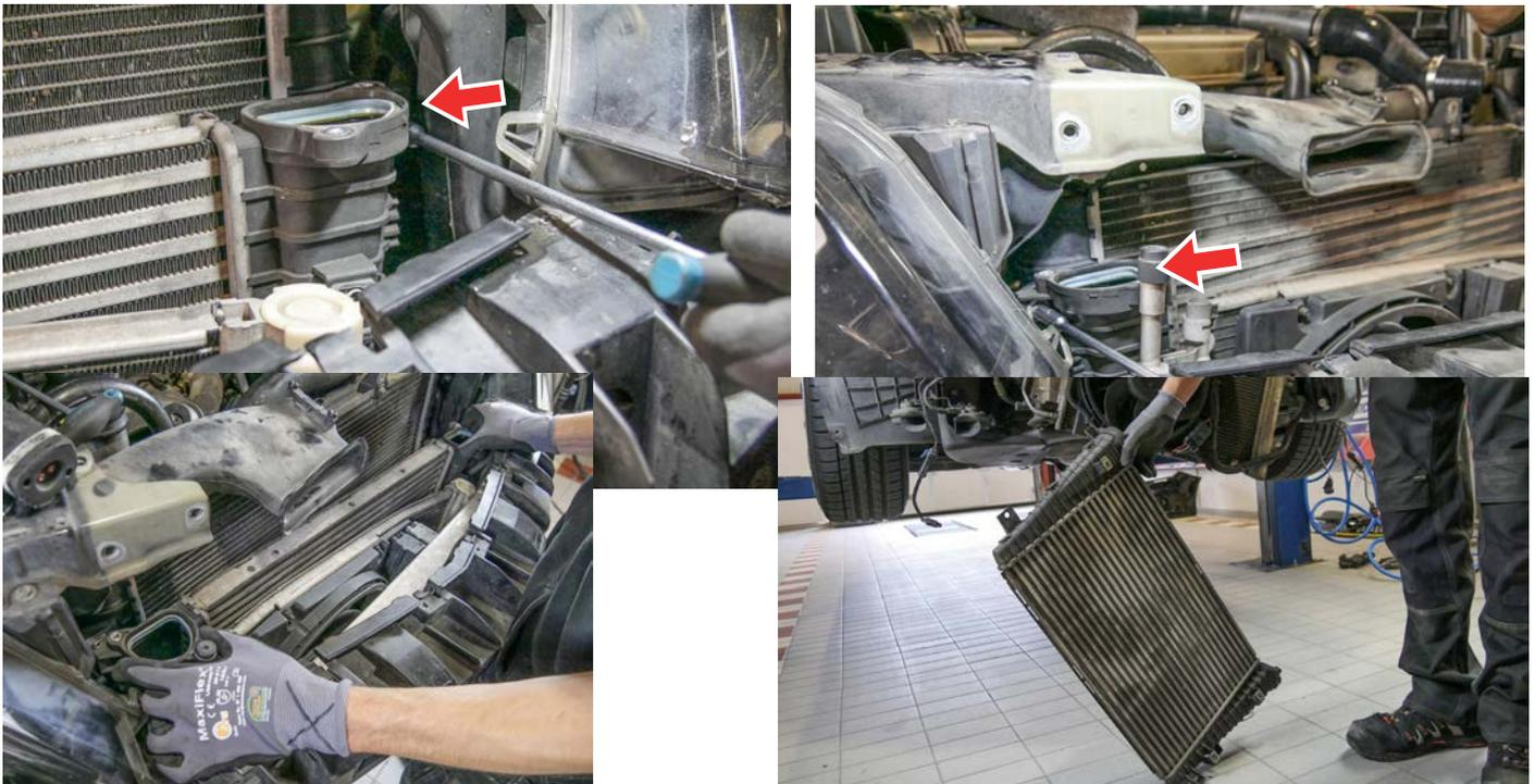
20. Please attach the air cooler again with the supplied kit (bracket) at the water cooler, because the HF-series intercooler it mounted in front of the air cooler.
