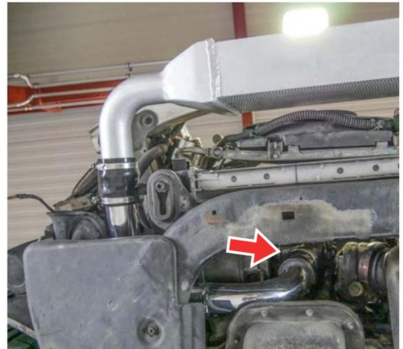
27. Now you can mount the casted aluminium tube, which is connected from the intercooler on the map sensor to the throttle.
