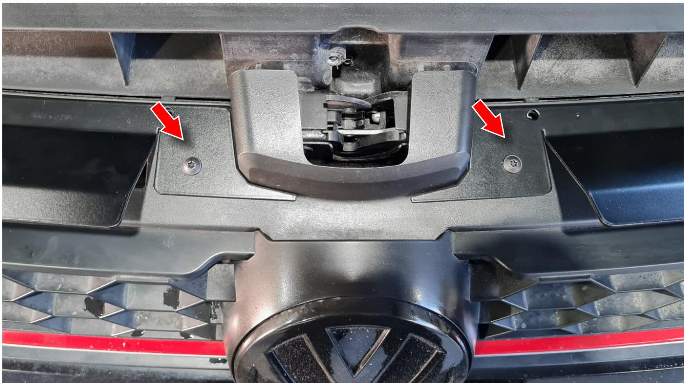
3. Mark the areas to be cut out using a permanent marker and then remove the radiator grille according to the manufacturer's instructions.
