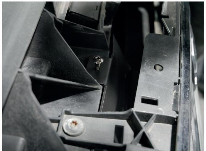
6. Once you have fixed both shields, you can fix the upper lock carrier cover with the previously removed plastic rivets.
