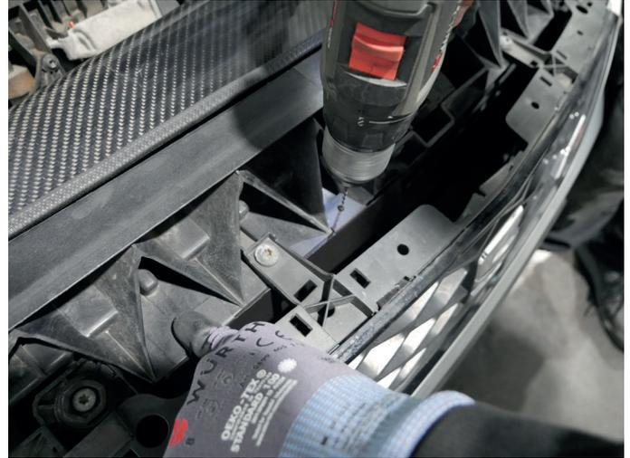
5. If you have drilled the two holes of the corresponding aircollector shield, you can fix the shield to the front mask with the supplied coarse thread screws. Repeat the steps accordingly for the other side.
