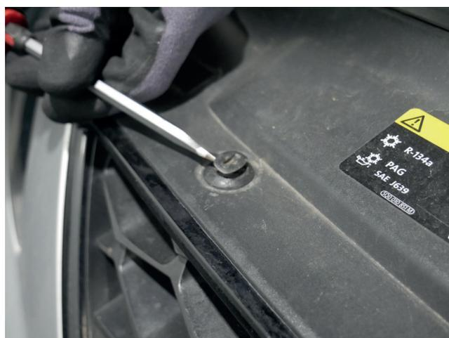
2. Gently pull the back edge of the cover upwards to remove the top cover of the lock carrier from the vehicle.
