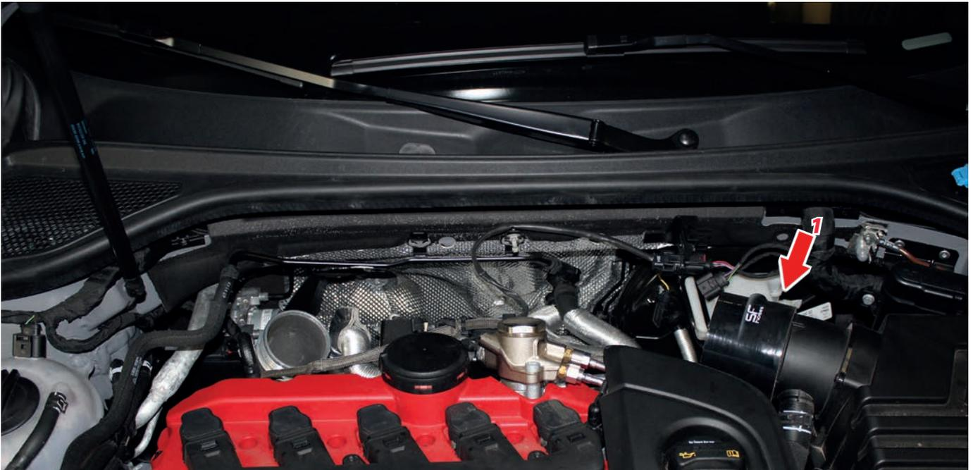
9. Place the HF-Series Air Intake as shown in the hump hose and tighten the hose clamps securely so far that you can rotate the intake still and adjust the position.
