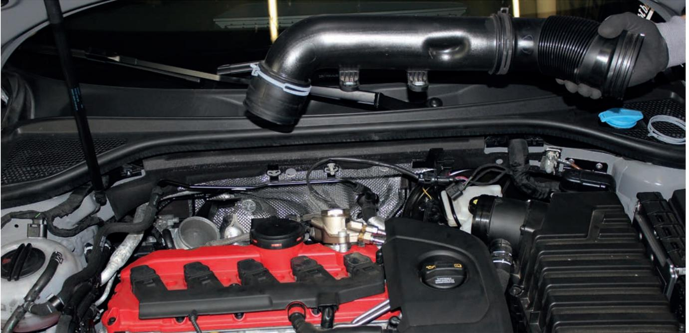
7. Now pre-assemble the **hump hose (1)** together with the two corresponding hose clamps on the air filter box connection.
