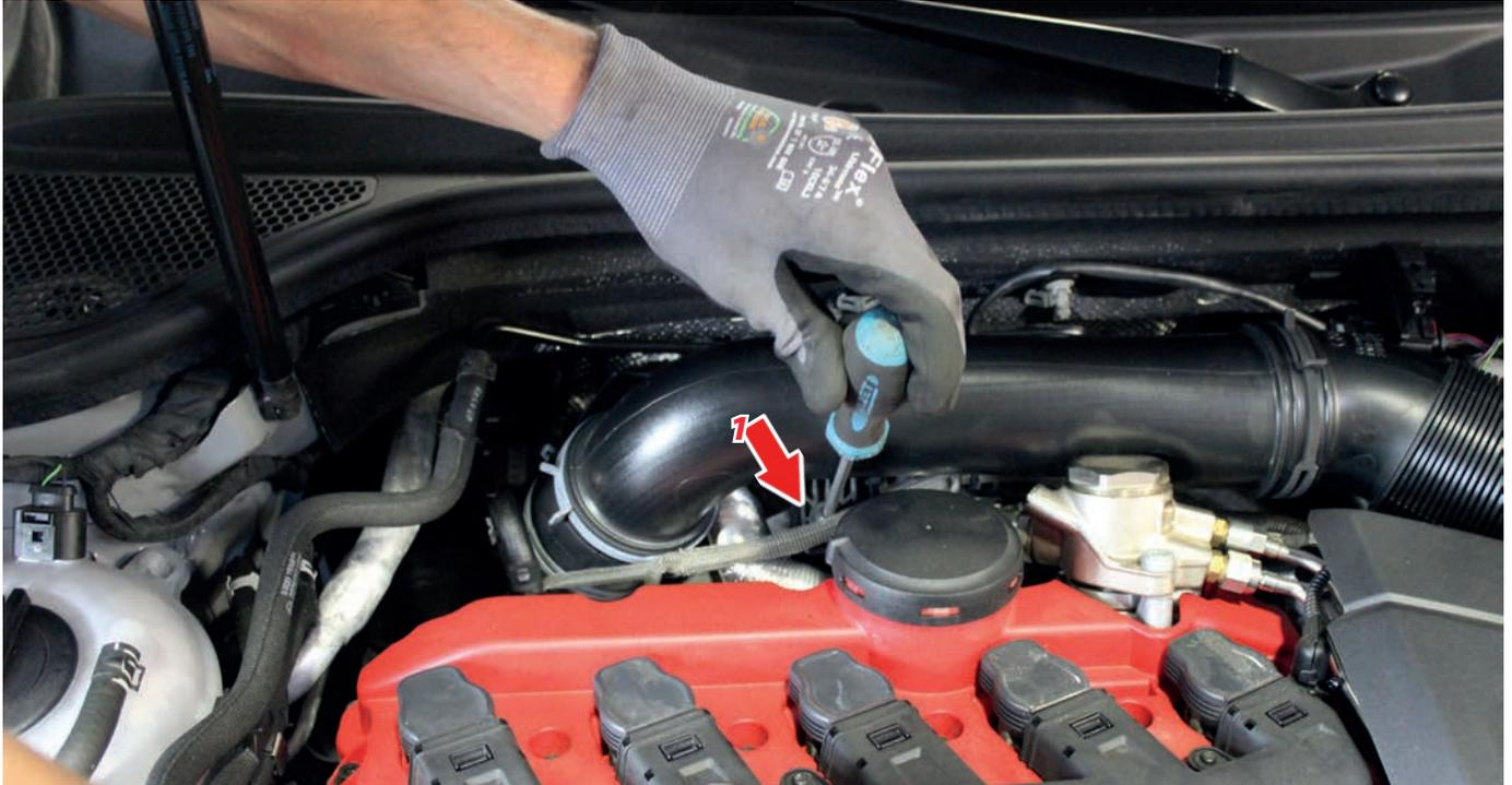
3. Do the same with the **T 30 - screw (2)** right behind the fuel pump. Again, tact is needed. If you have, use a magnet holder for help.
