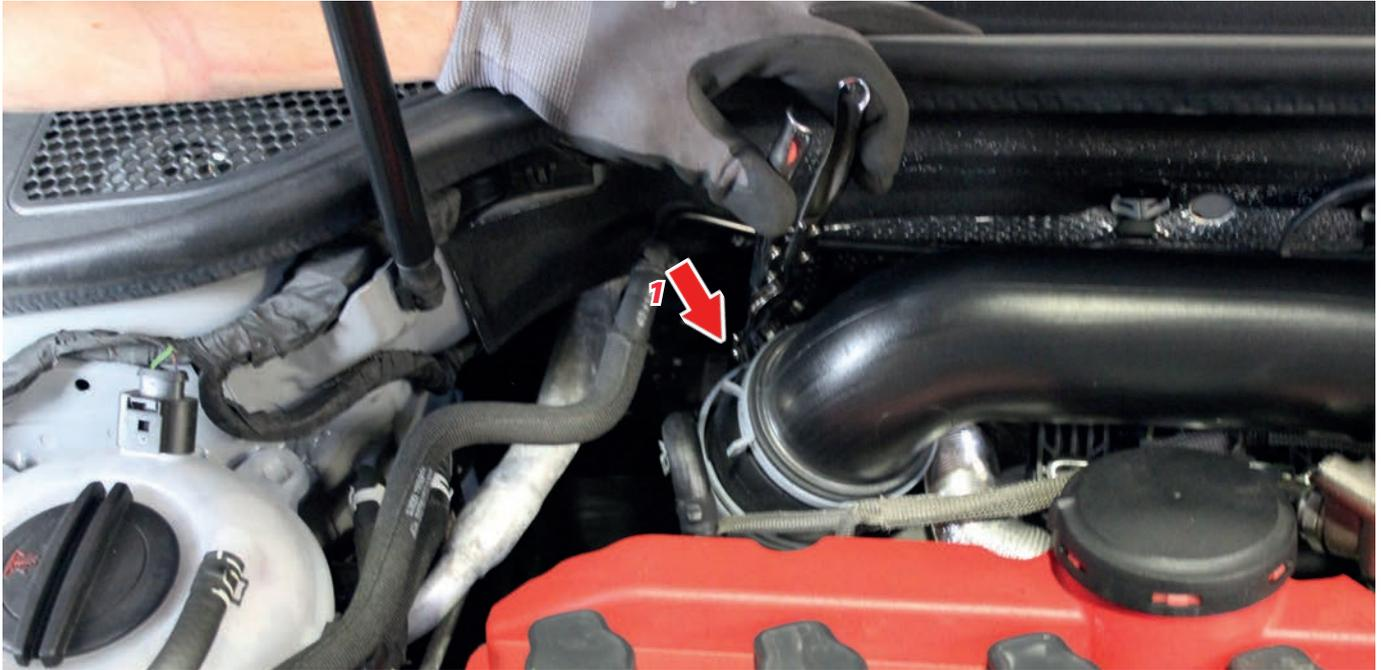
5. Now open the **hose clamp (2)**, which is located at the end of the intake pipe to the air filter box. Then pull the original intake pipe from the air filter box.
