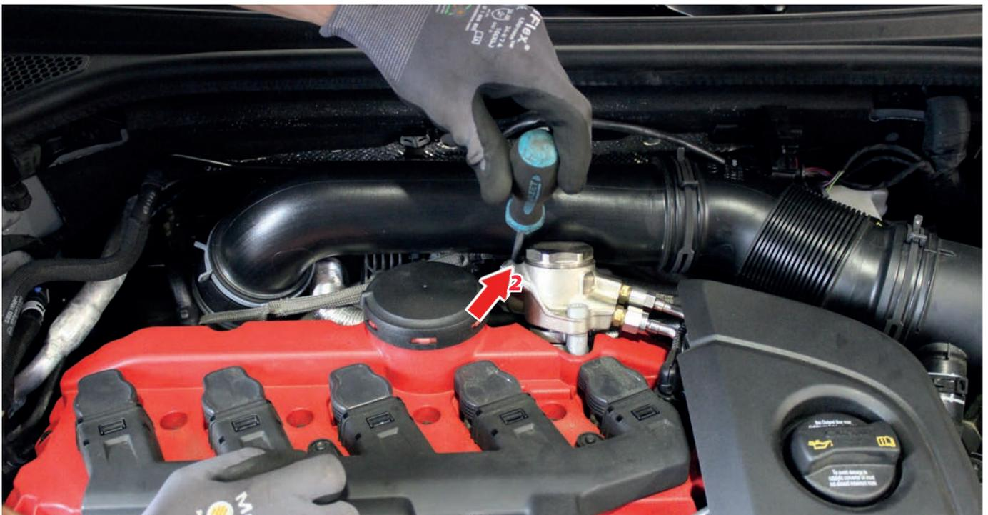
4. Loosen with a hose clamp-forceps or alternatively a water pump pliers **the hose clamps (1)** at the end of the intake pipe. Tighten the hose clamps so far from the connection that you can afterwards disconnect the intake pipe from the turbocharger.
