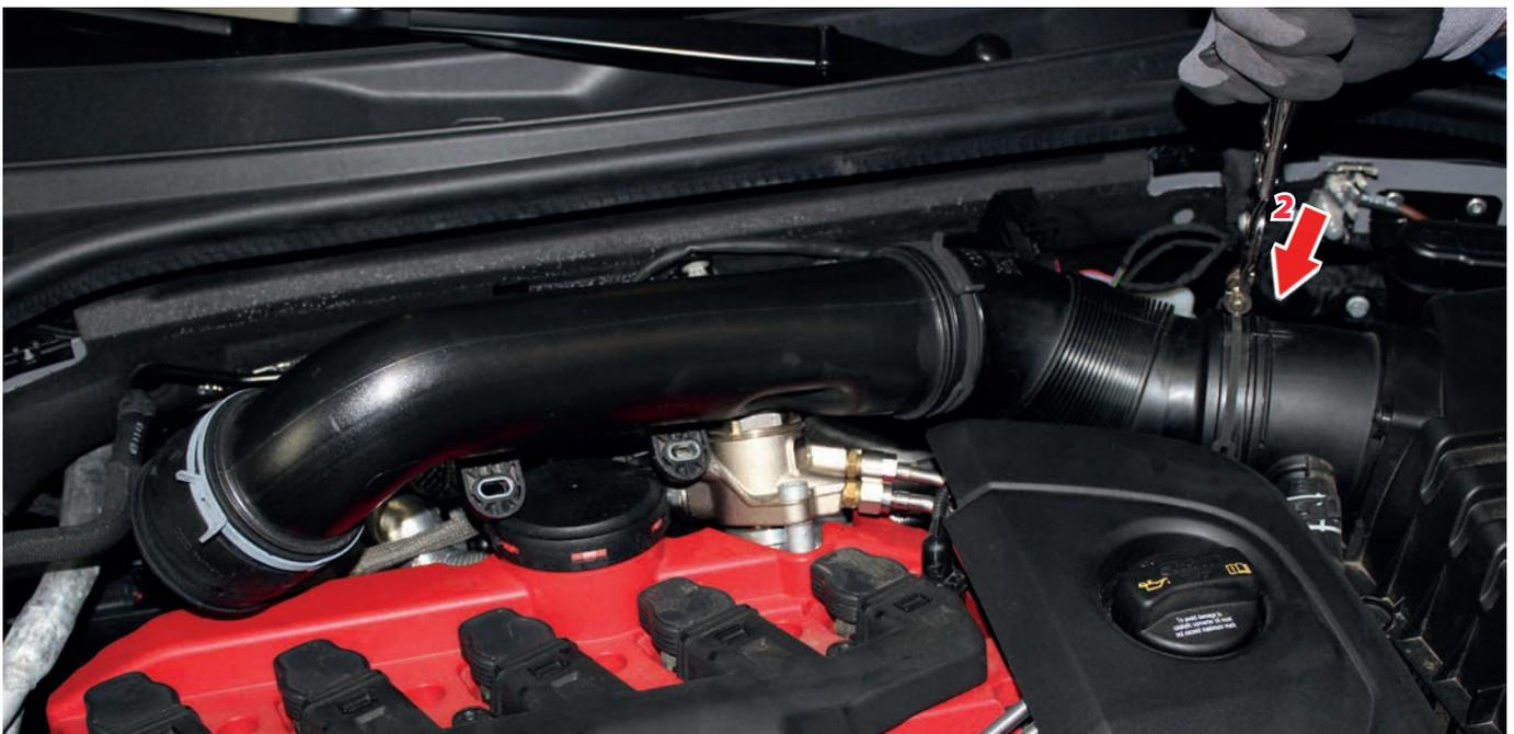
6. Remove now complete the original intake pipe from the engine compartment.
