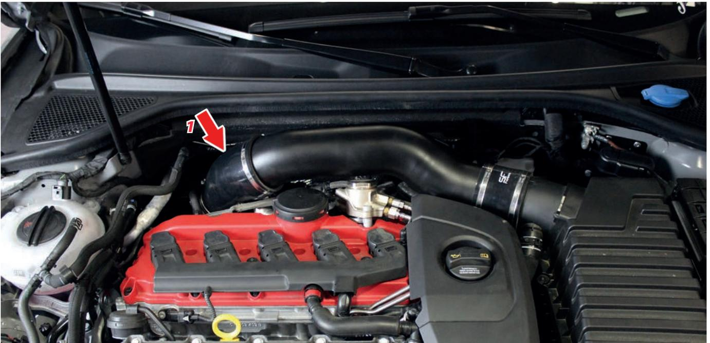
11. Check now again the correct position of the HF Series Air Intake, the silicone parts and the clamps. Unless strikes, scrubs, or interfere with the function of another component, tighten all clamps with a 7mm- spanner, alternatively with a ratchet and a corresponding nut or a T-handle.
