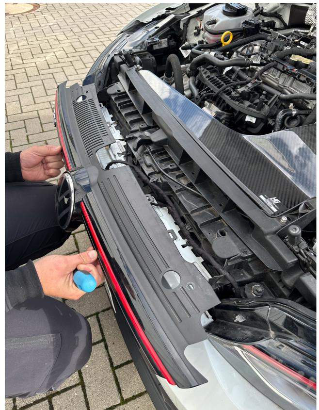
3. Remove the standard cable connections from the front grill.
