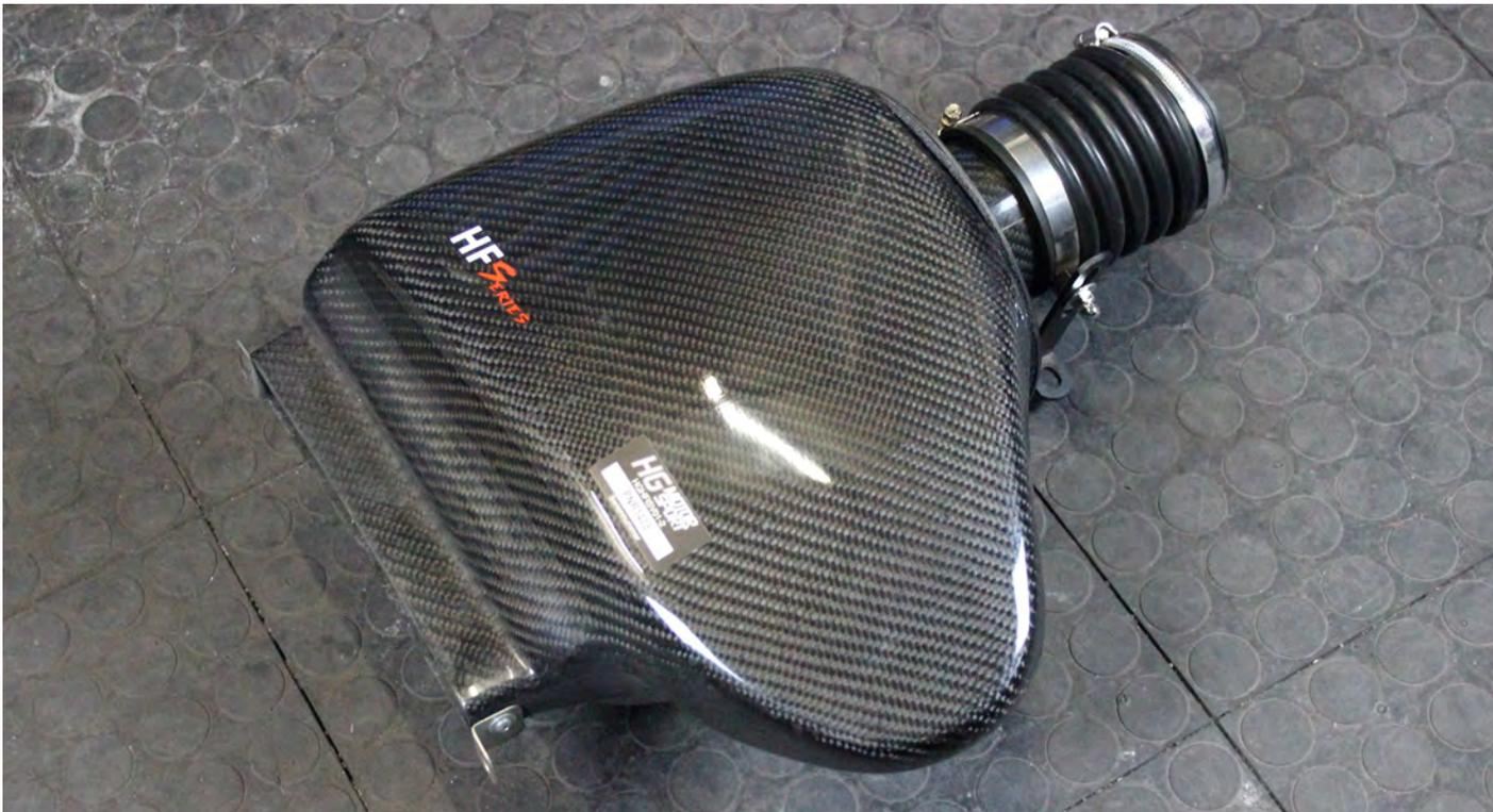
25. Press the vibration damper on the airbox together lengthwise so that you can place the airbox between the intake pipe and the air intake in the lock carrier. Then tighten the retaining brackets to the lock carrier or air intake using the T25 Torx screws.
