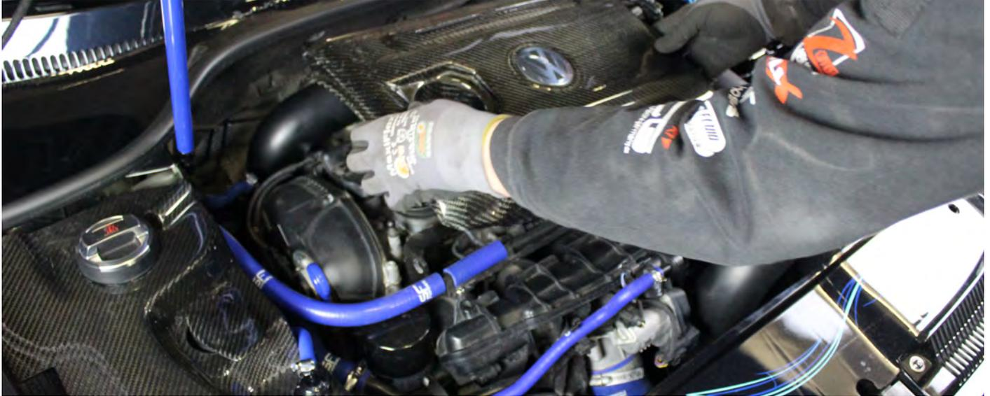
3. Remove the cover of the air collector by gently prying off the **3 retaining clips (1)**.
