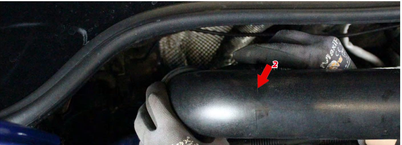
17. Prepare the HF-Series intake pipe so that you can fix the silicone reducer with clamps and the silicone connector on the intake pipe with a clamp.
