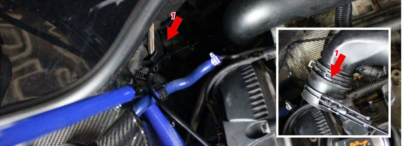
16. Remove the **crankcase ventilation hose (2)** by pressing the clamping ring together.
