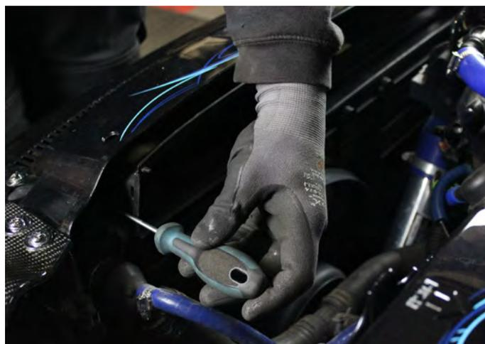
14. Remove the T30 Torx screw on the back of the intake pipe. **(ATTENTION: Caution!!! If you do the conversion just after you have still been driving the vehicle, this area can be very hot!)**
