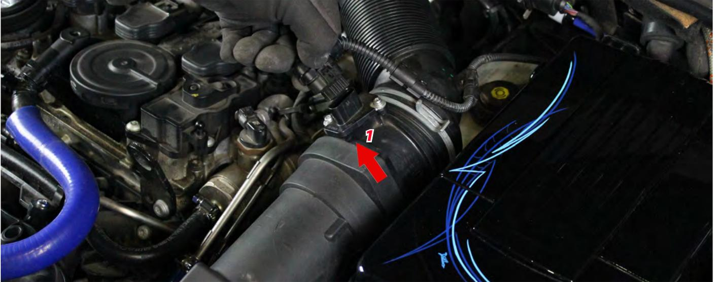
5. Open the **hose clamp (2)** between the mass air flow sensor and the intake pipe using hose clamp pliers.
