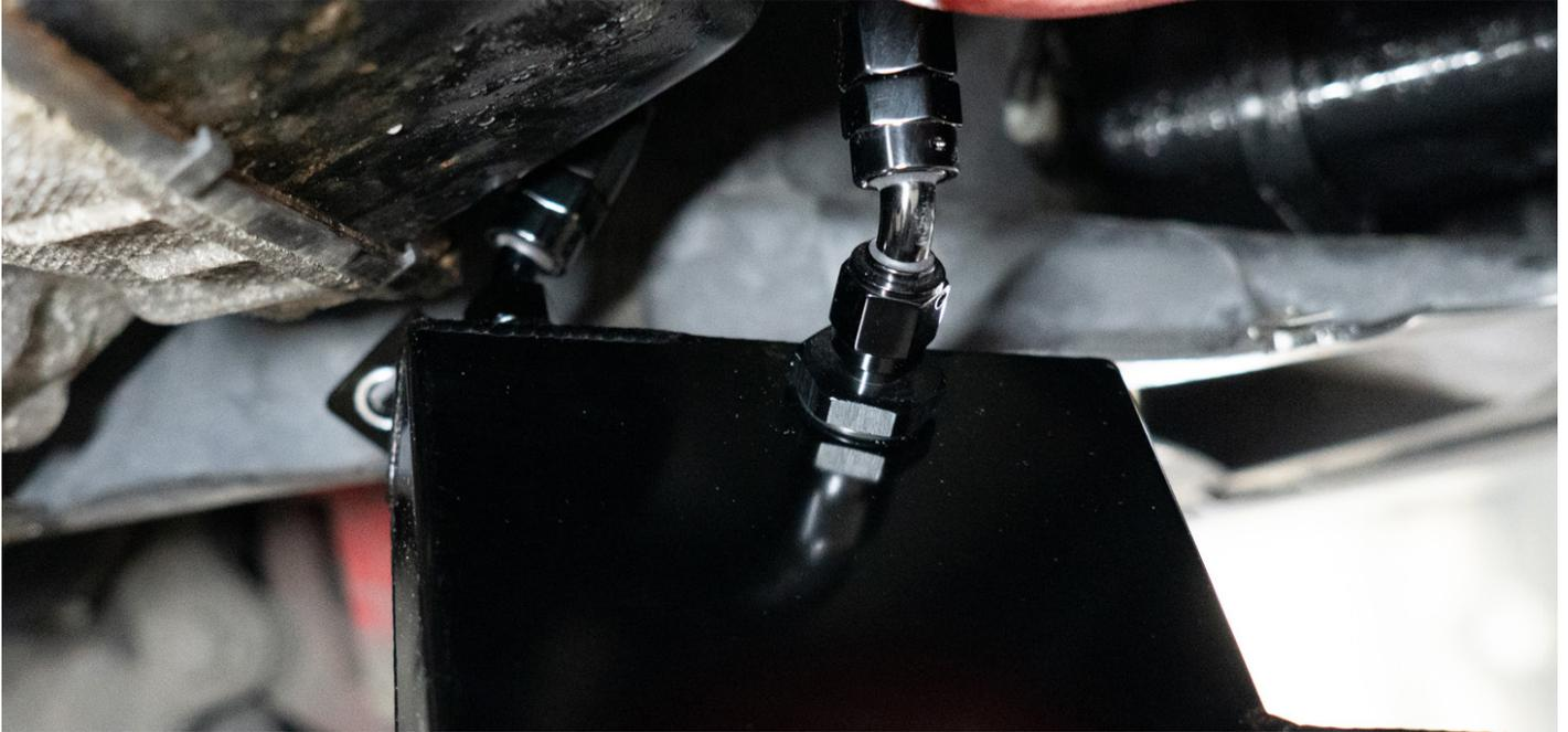
12. Mount the CatchCan next to the right intercooler hose, using two screws (M6 & M8) as shown in the pictures.
