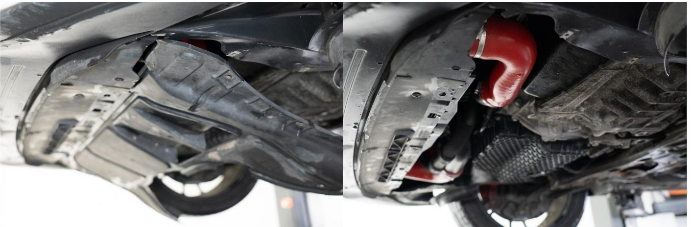
10. Guide the first hose from the turboinlet towards the underbody and mount it on the top of the catchcan.
