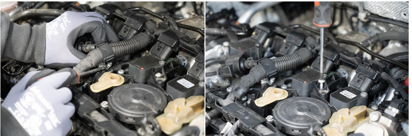
2. Disassemble the crankcase ventilation pipe as shown in the pictures.
