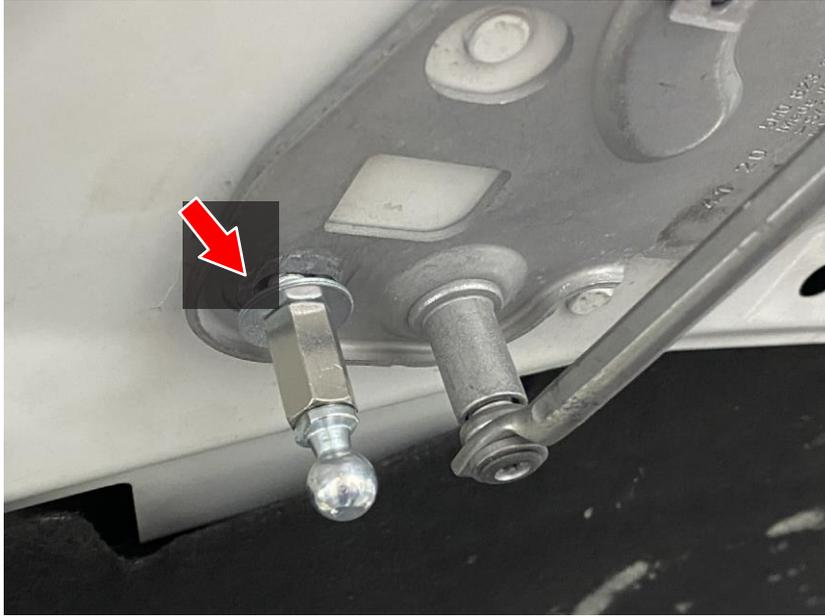
4. Mount the HG Motorsport hood lift to the existing ball head (right above the coolant reservoir) (picture 1) & to the previously mounted ball head on the hood (picture 2).
