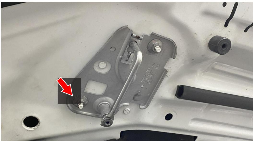
3. Mount the supplied threaded ball head, together with the washer (see picture) and tighten it with 20Nm (10mm nut).
