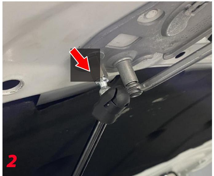
5. CAUTION! Remove the standard hood bracket before closing the hood to avoid damage to the vehicle.
