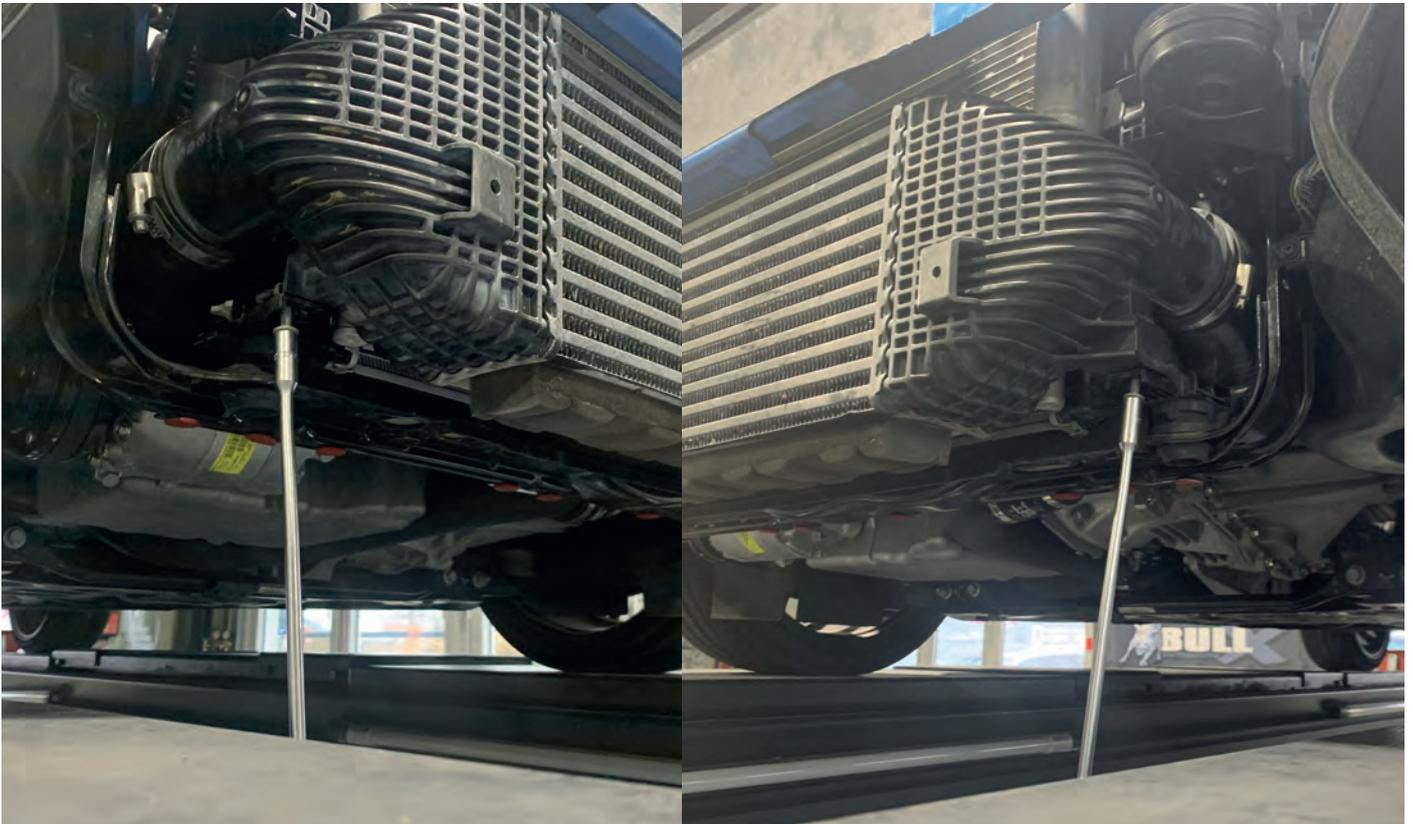
4. Loosen the hose clamps on the charge air cooler with a 7mm nut.
