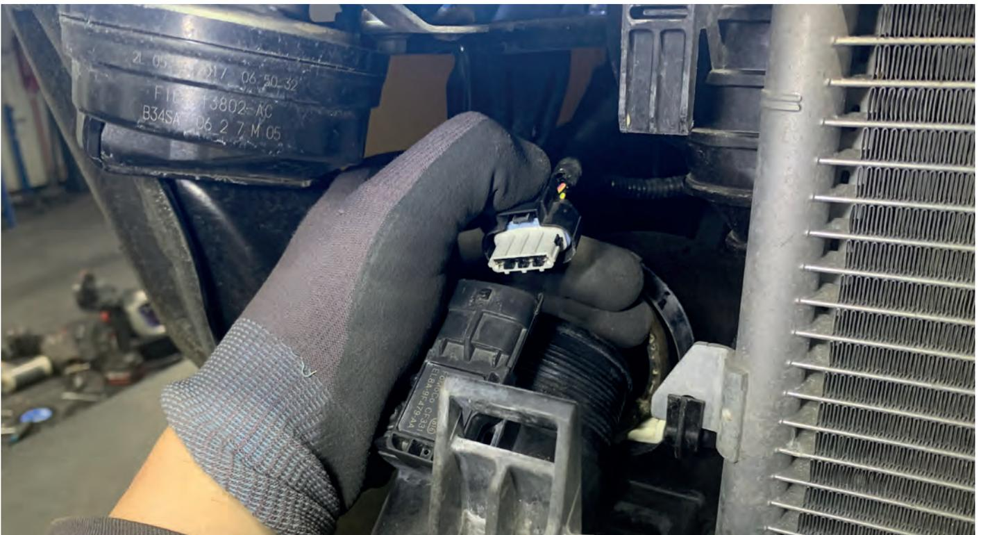
*Note: Depending on the mileage of your vehicle, the clamps and the charge air hoses may be more or less stuck. If necessary, use a larger flat-blade screwdriver or similar to remove the hoses from the charge air cooler. But do not damage the charge air hoses or the clamps, as you will continue to use them.*
