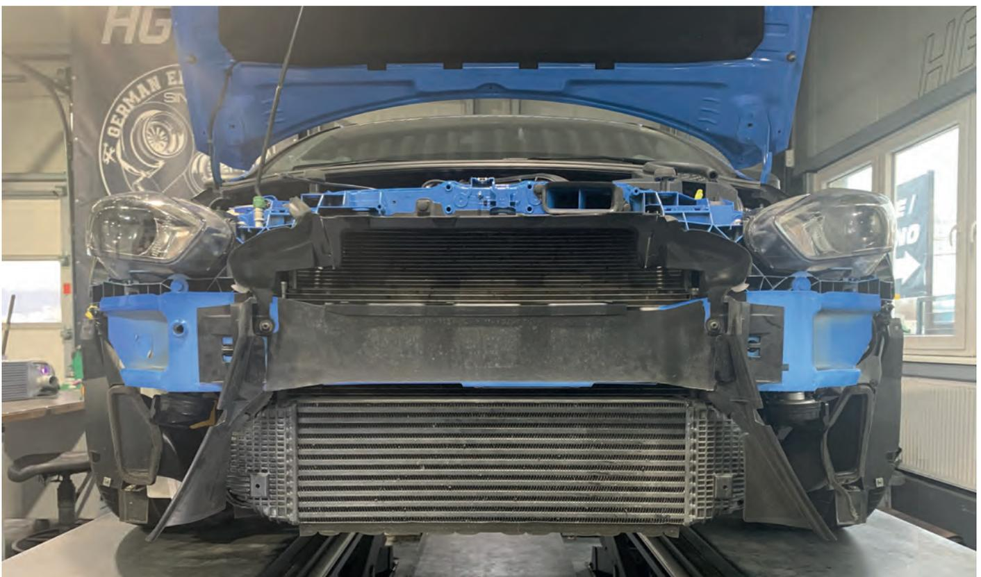
2. Disassemble the plastic cover with a TX-30 Torx screwdriver.
