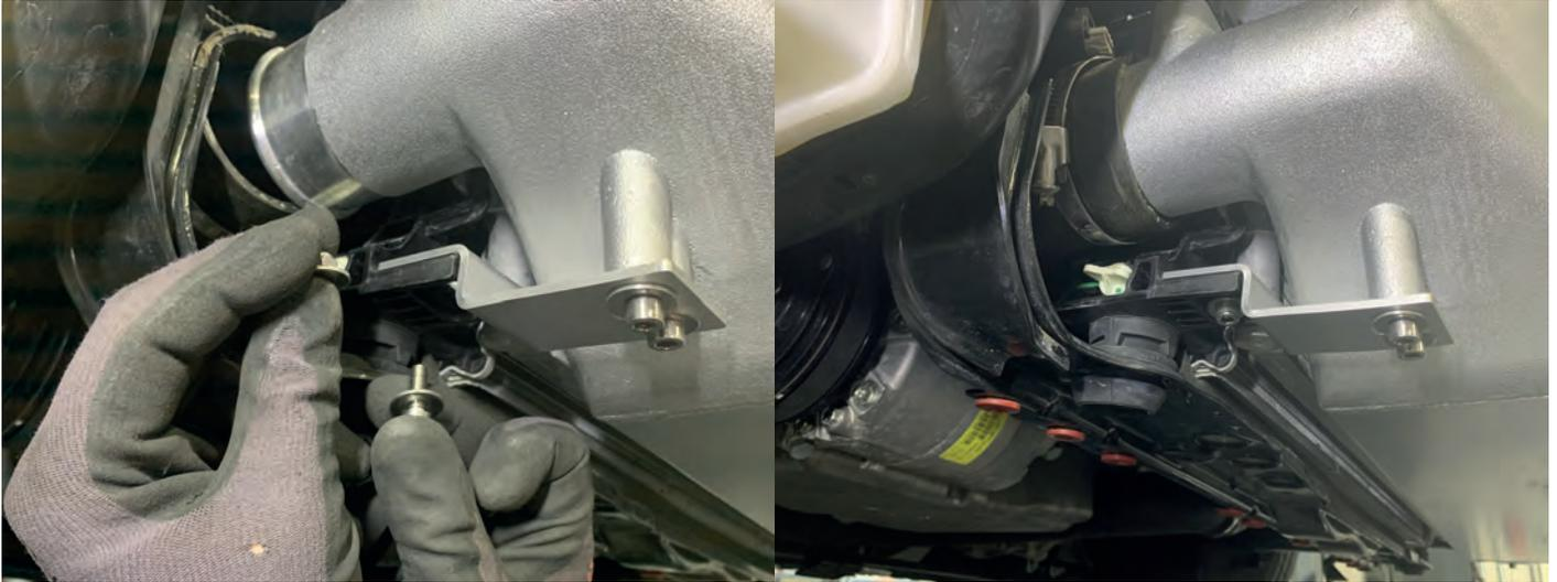
12. Now mount the charge air hoses on the charge air cooler & fasten them with the standard hose clamps.
