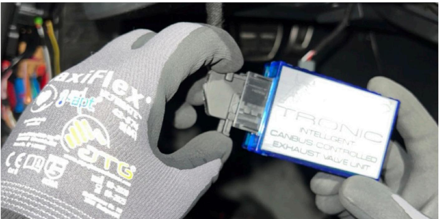
**From this point on, do not switch on the ignition under any circumstances, otherwise a short circuit may occur on the cable to the solenoid valve.**
