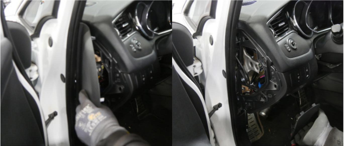
2. The power supply (+) of the Bull-X-Tronic, take off at the fuse box(MF35) top right.
