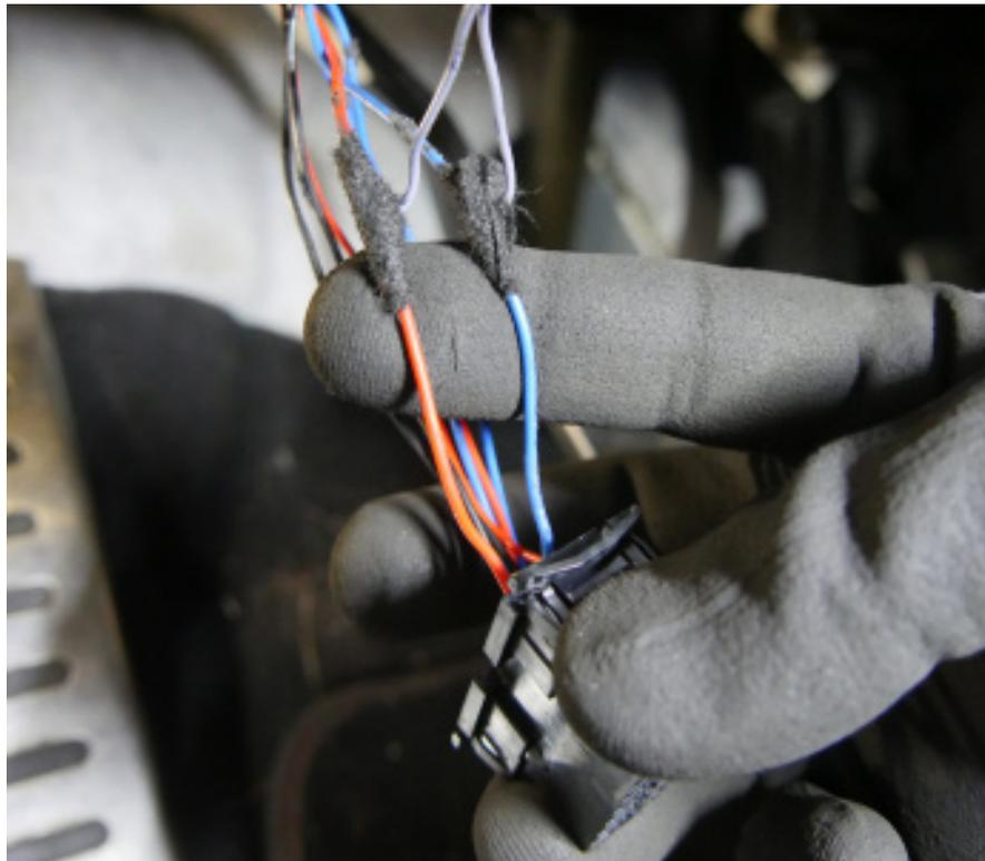
4. Connect the ground cable as shown in the picture. This point is located in the driver's footwell, on the left side of the body.
