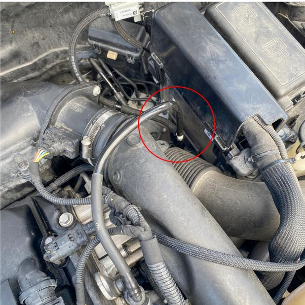
2. Now connect the non-return valve and the magnet valve to the vacuum hose.
