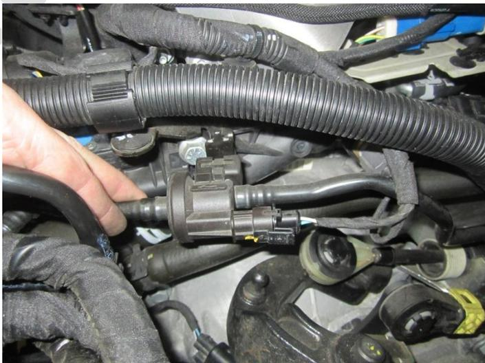
**Step 8:** Place the extraction tool on the ball head as shown.
