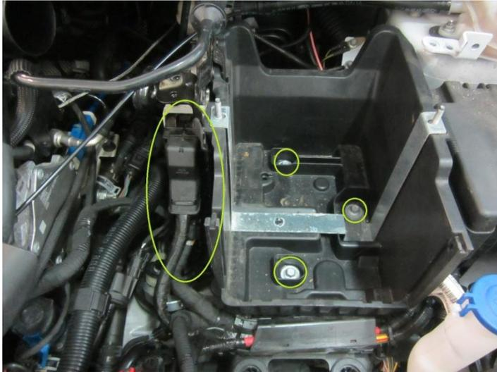
**Step 6:** Carefully lever out the shift cable using a screwdriver.
