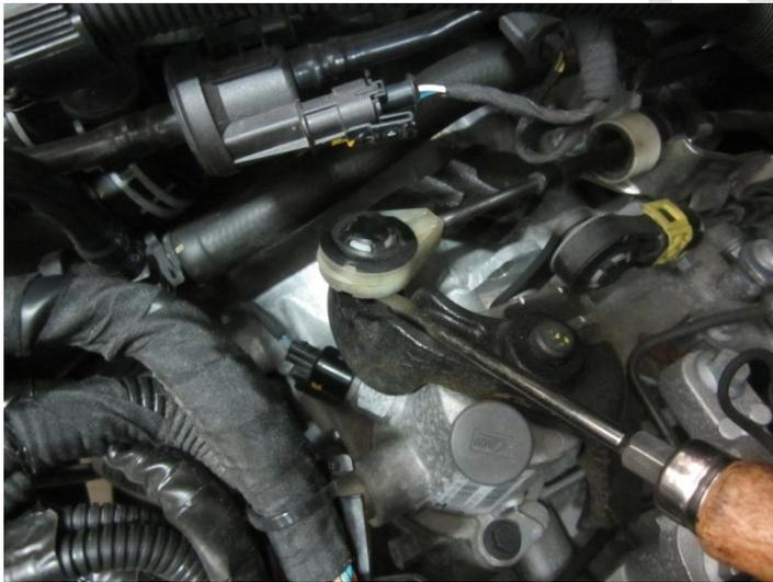
**Step 7:** Pull the clock valve upwards out of the holder and place it below the holder to make room for the extraction tool.
