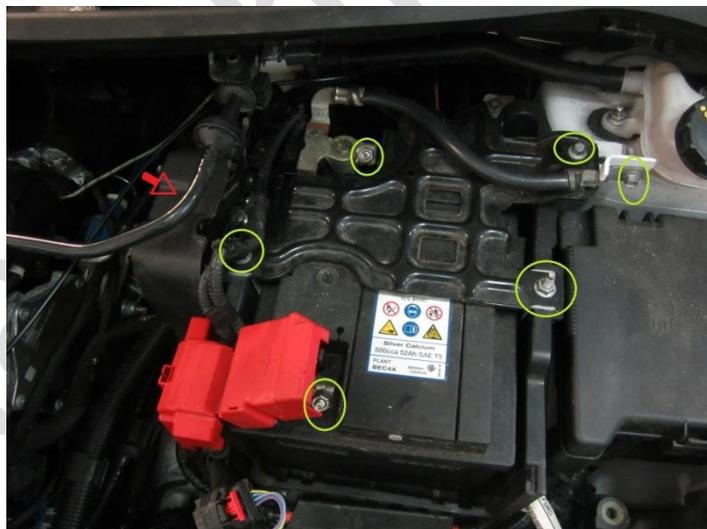
**Step 5:** Unscrew the three screws and disconnect the two connectors of the control unit. Now remove the battery box together with the control unit.
