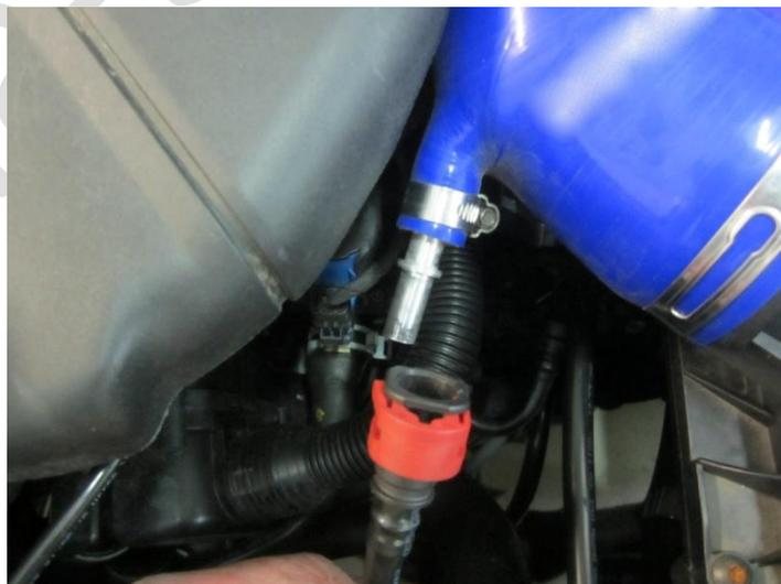
**Step 3:** Disconnect the plug of the mass air flow sensor. Loosen the intake manifold towards the rear and remove the airbox by pulling it upwards.
