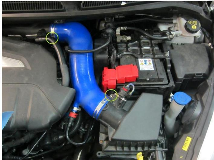
**Step 2:** Disconnect the vent connection. Now remove the intake hose and put it aside.
