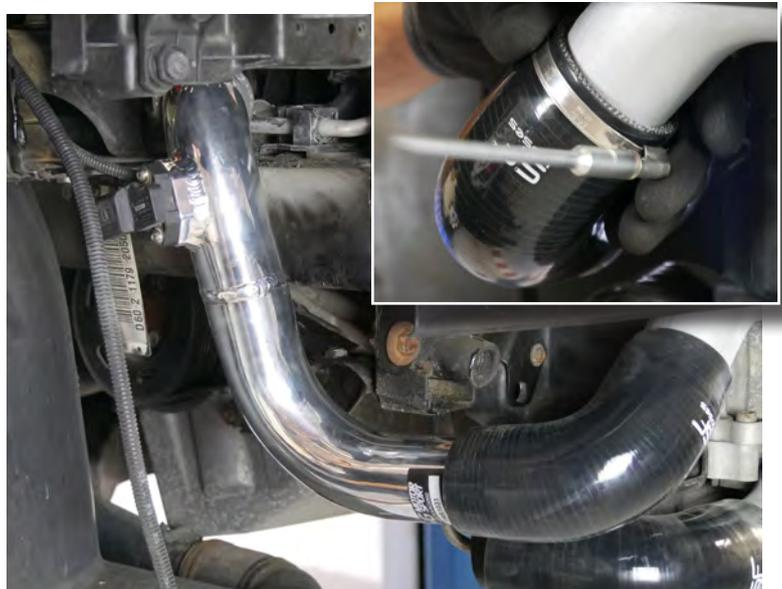
12. The lower pressure pipe is separated from the original silicone hose and replaced with the new pressure pipe from HF-Series. Please note the holder next to the oil pan.
