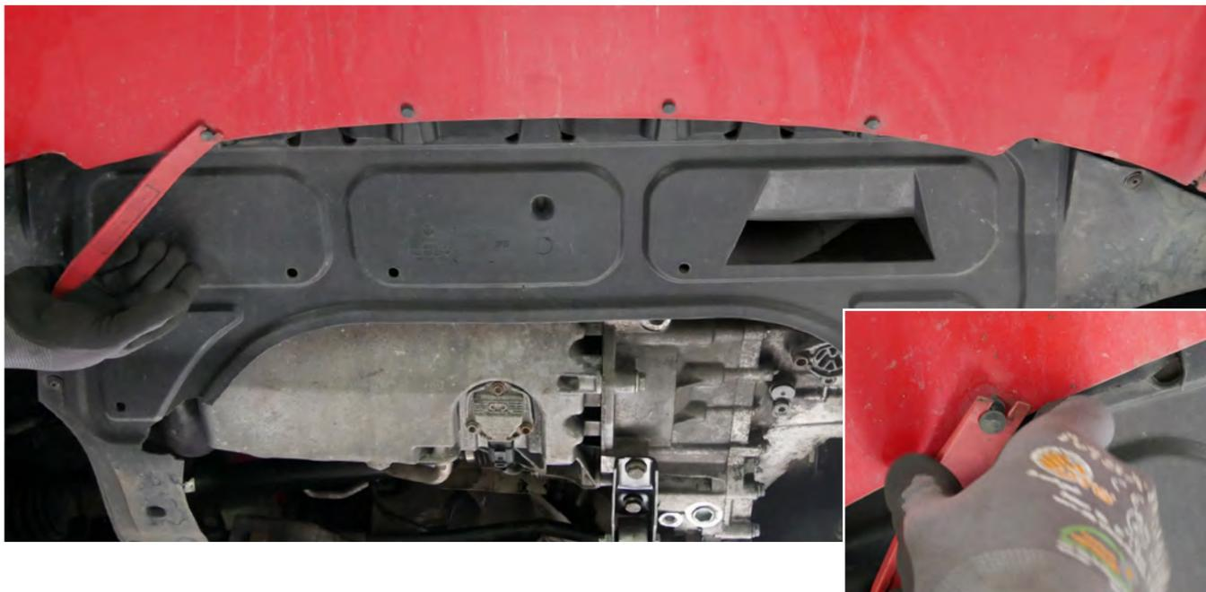
3. The wheel arch liners are fixed with 4 screws. Two more are there for the bumper and underbody protection. Please unscrew all screws. Now the remaining splash guard can also be removed from the underbody.
