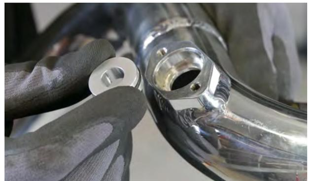
11. Install the MAP sensor from the original intercooler together with the supplied aluminium gasket and mounting material in the HF-Series pressure pipe. This pressure pipe is attached to the upper intercooler connection with an SF-Hoses silicone hose and runs from there to the intake manifold. In the course of this, the connector for the MAP sensor is reconnected and the hoses are fitted with the appropriate hose clamps.
