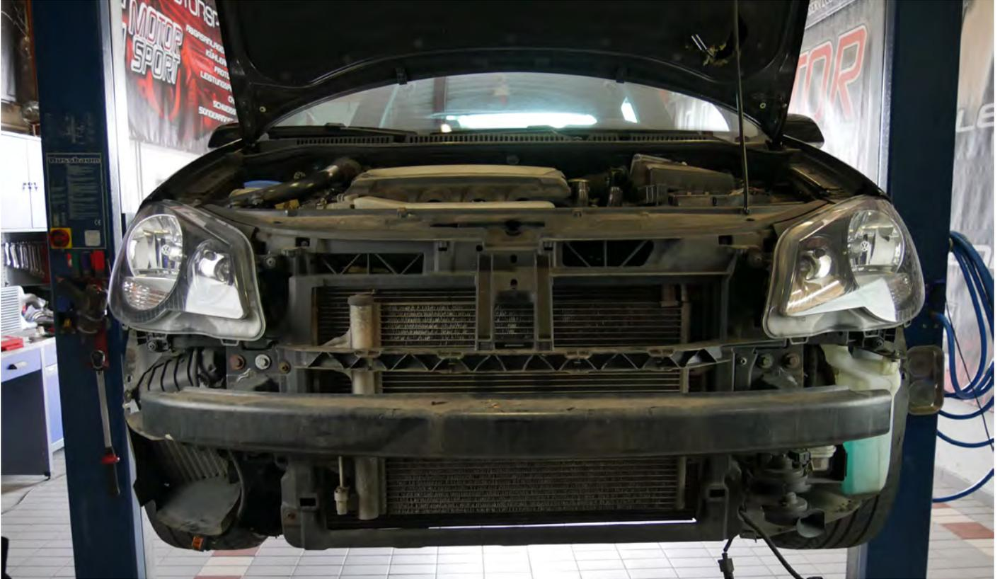
7. After the bumper has been removed, all parts of the intercooler can be removed. This includes the air duct, which is clipped in place, the connector behind the manifold and the underpressure hose.
