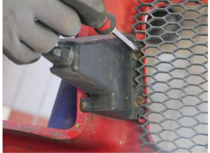
13. The bumper must now be modified so that it can be reassembled. The first step is to remove the grille. On the left side (in the direction of travel), only the bumper holder must be unscrewed, then the grille can be reinserted.
