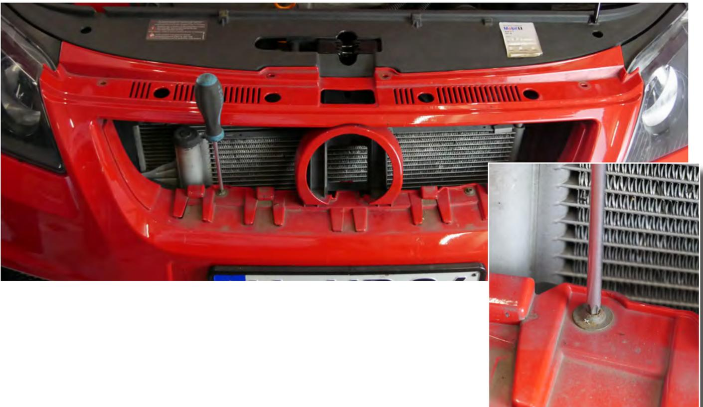
6. Remove the bumper towards the front. Please note the cable connection to the fog lights.
