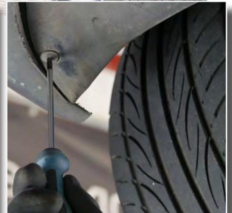
2. Remove the plastic rivets to the bumper as well. Now you can remove the underbody protection.
