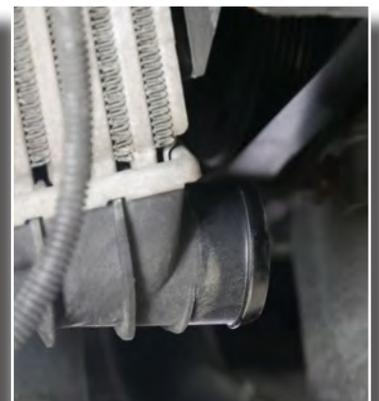
8. Now open the hose clamp on the intake manifold and pull off the silicone hose. The intercooler is screwed at 3 points. Loosen all screws and remove the intercooler.
